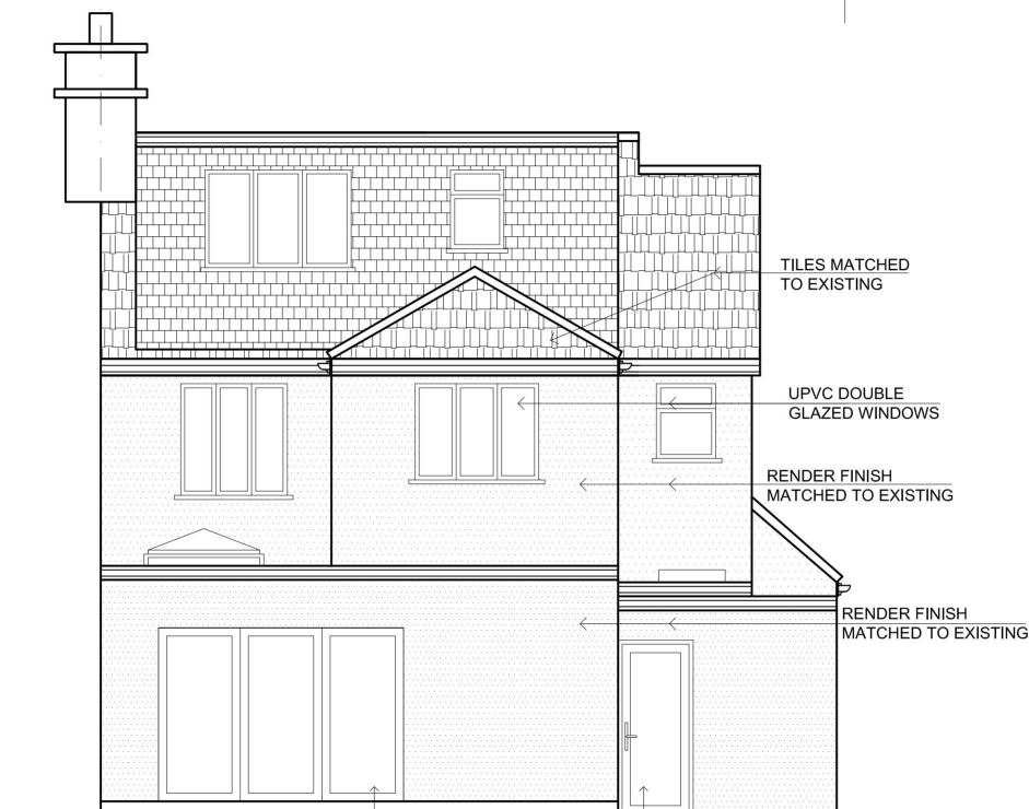
EXISTING REAR ELEVATION
