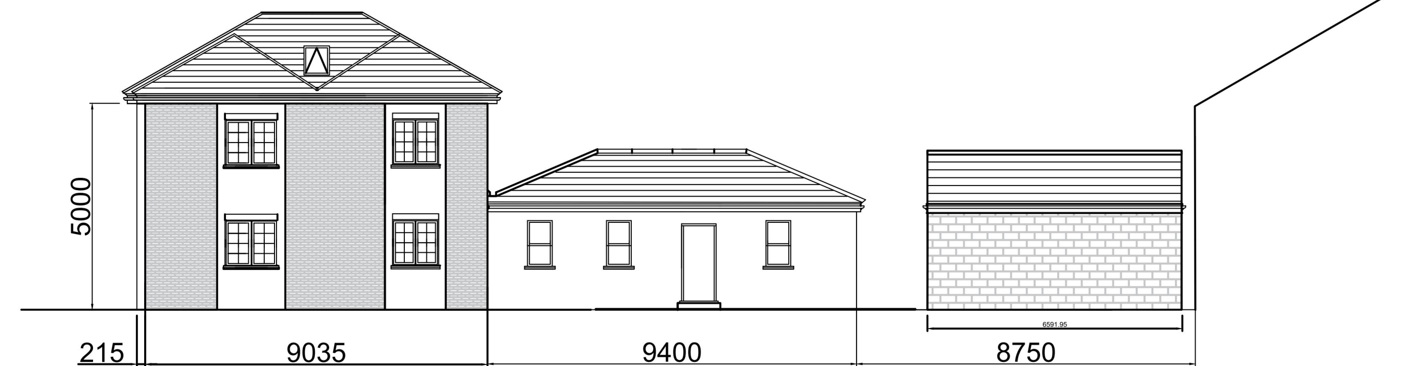
PROPOSED REAR ELEVATION
