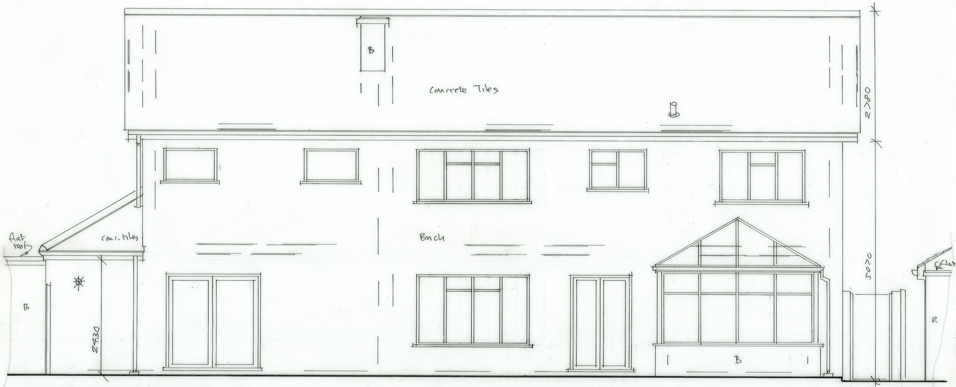
EXISTING REAR ELEVATION 1:50
