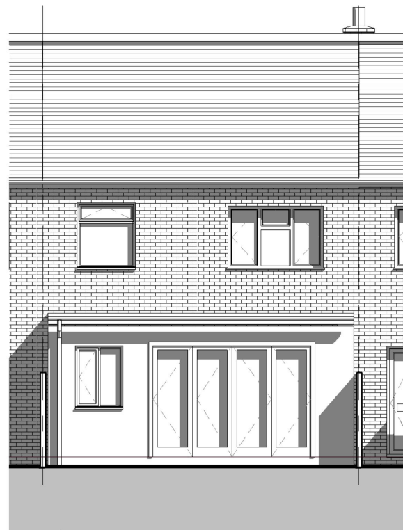
2 Existing Rear Elevation 1 : 100
