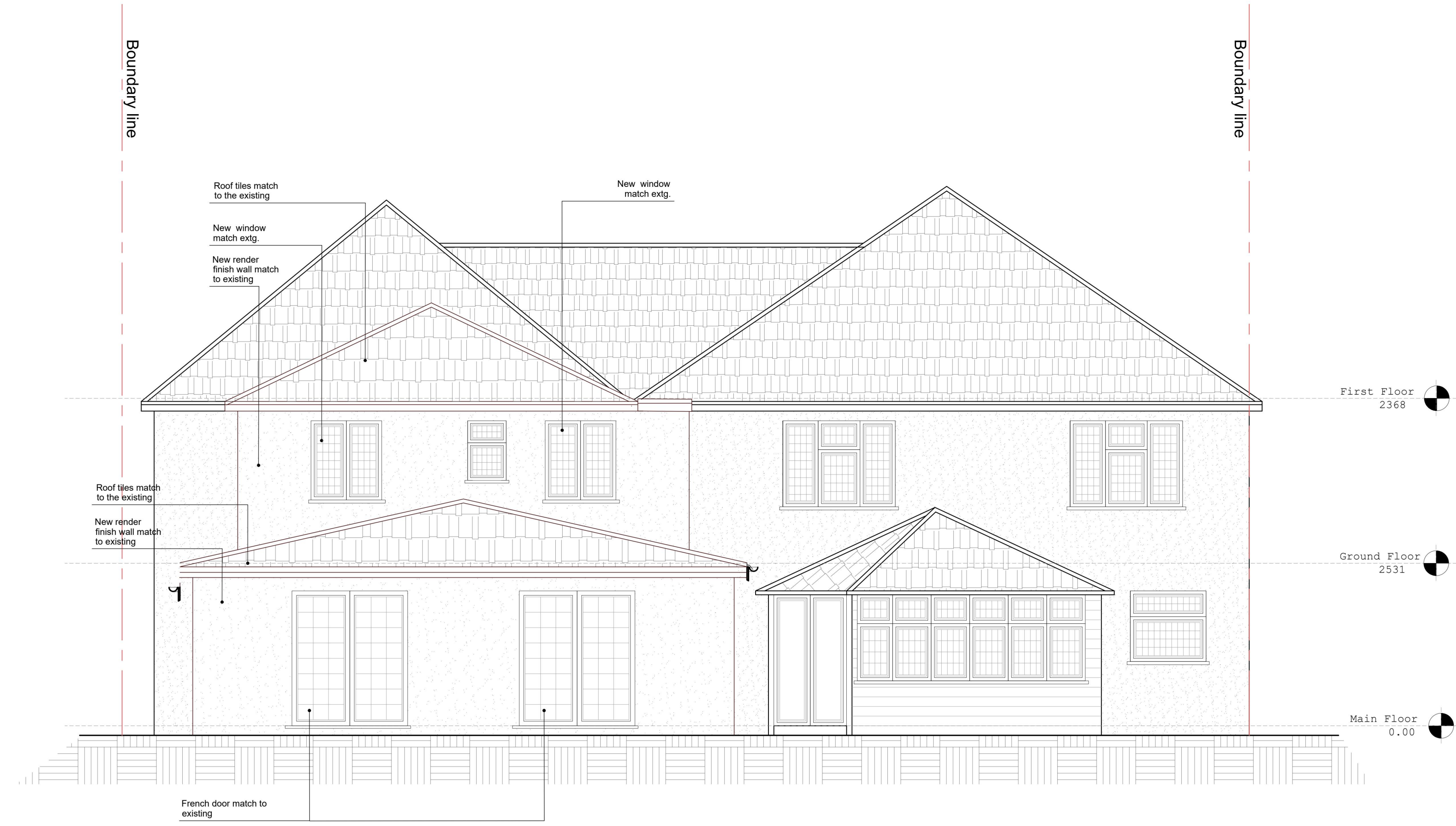
PROPOSED REAR ELEVATION SCALE 1:50
