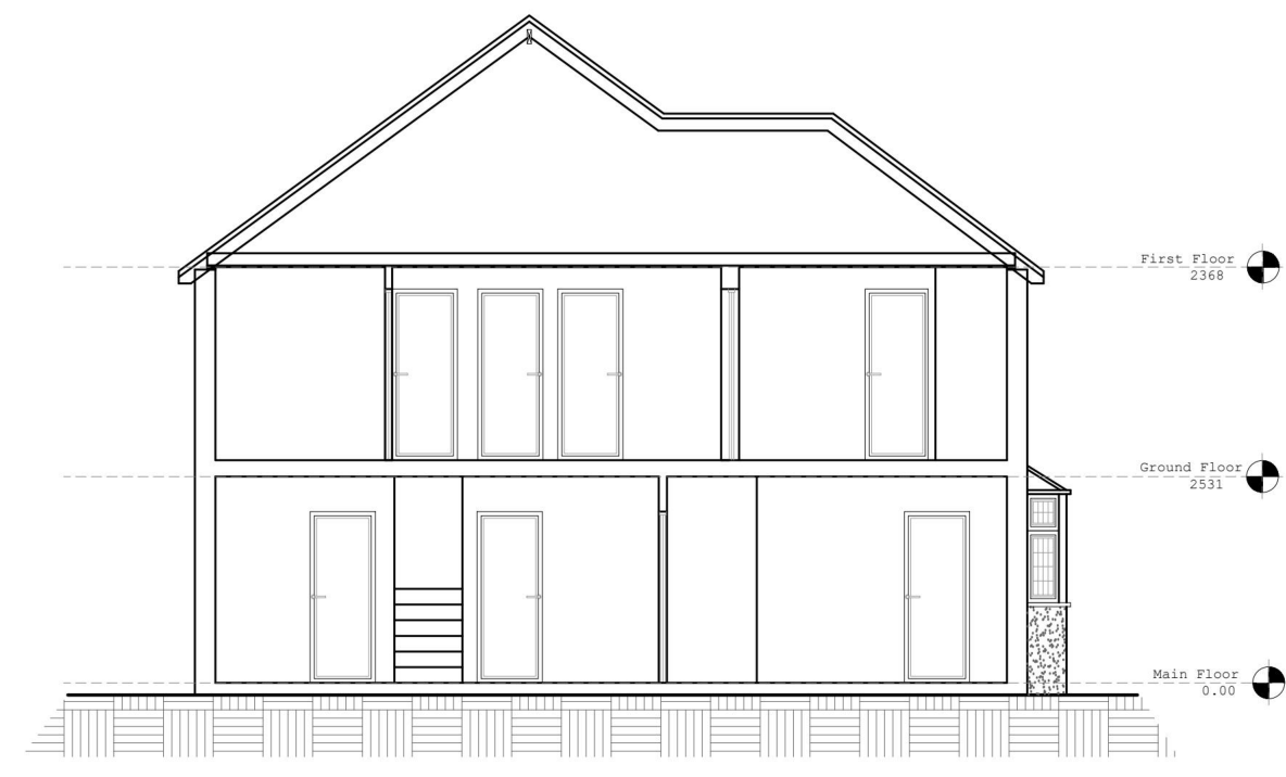
EXISTING SECTION AA SCALE 1:100
