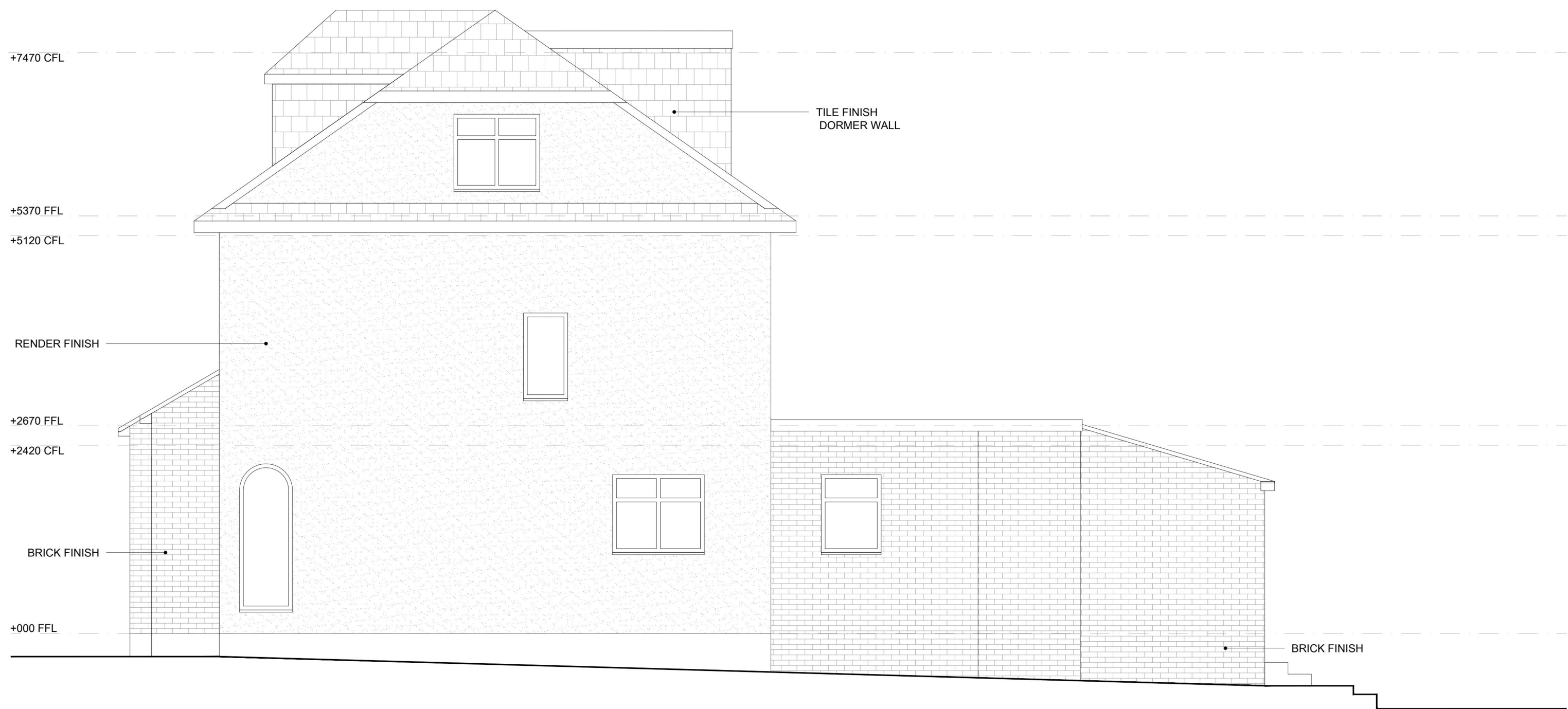
PROPOSED Right Elevation scale 1:50 @ A1 | 1:100 @ A3
