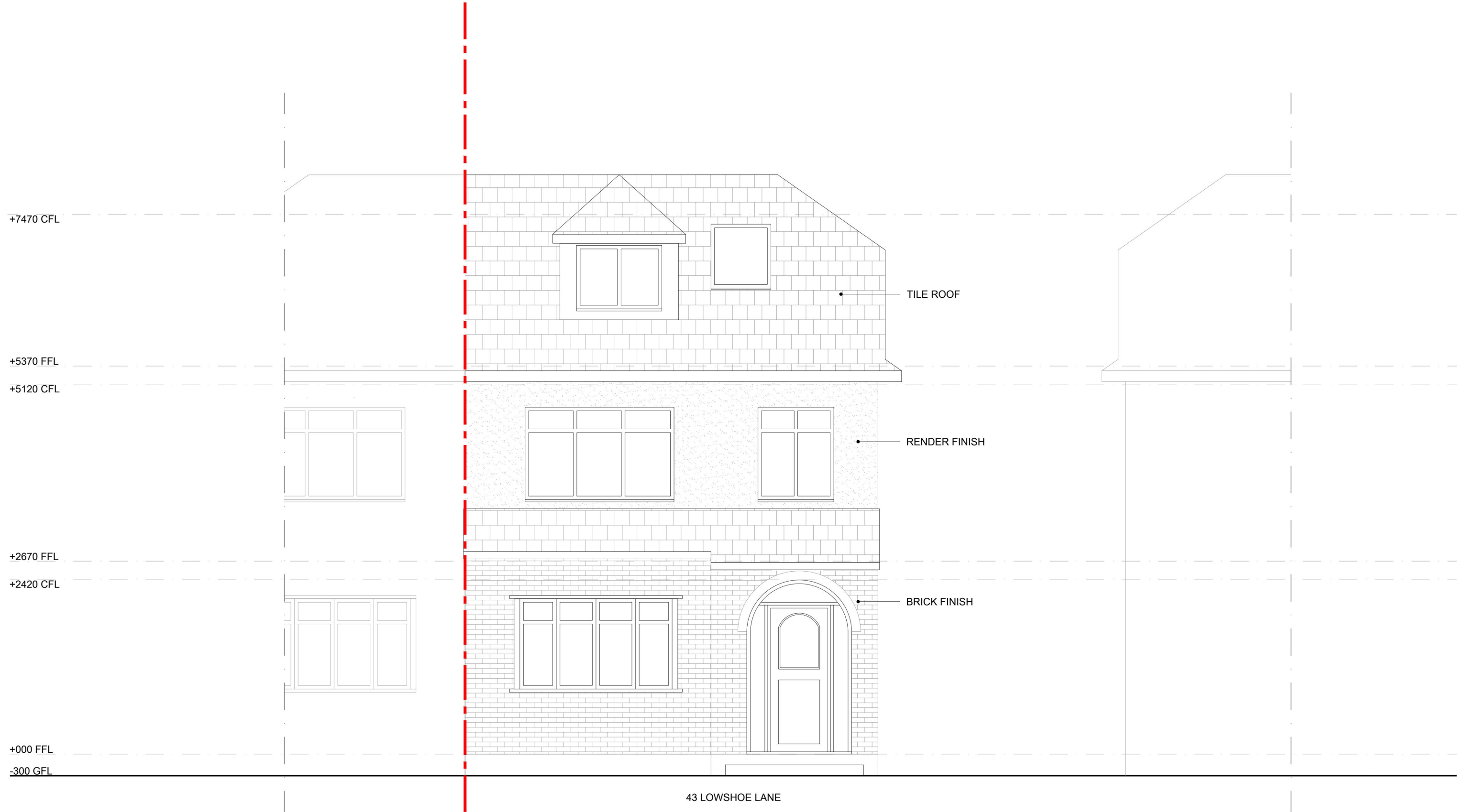
PROPOSED Front Elevation scale 1:50 @ A1 | 1:100 @ A3
