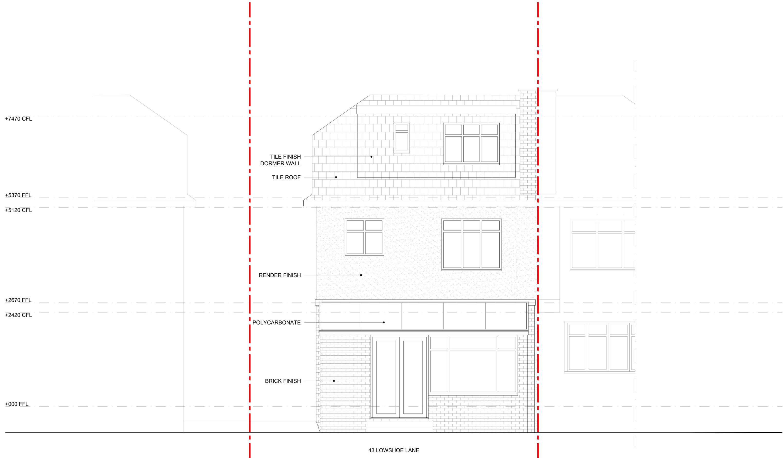
PROPOSED Rear Elevation scale 1:50 @ A1 | 1:100 @ A3
