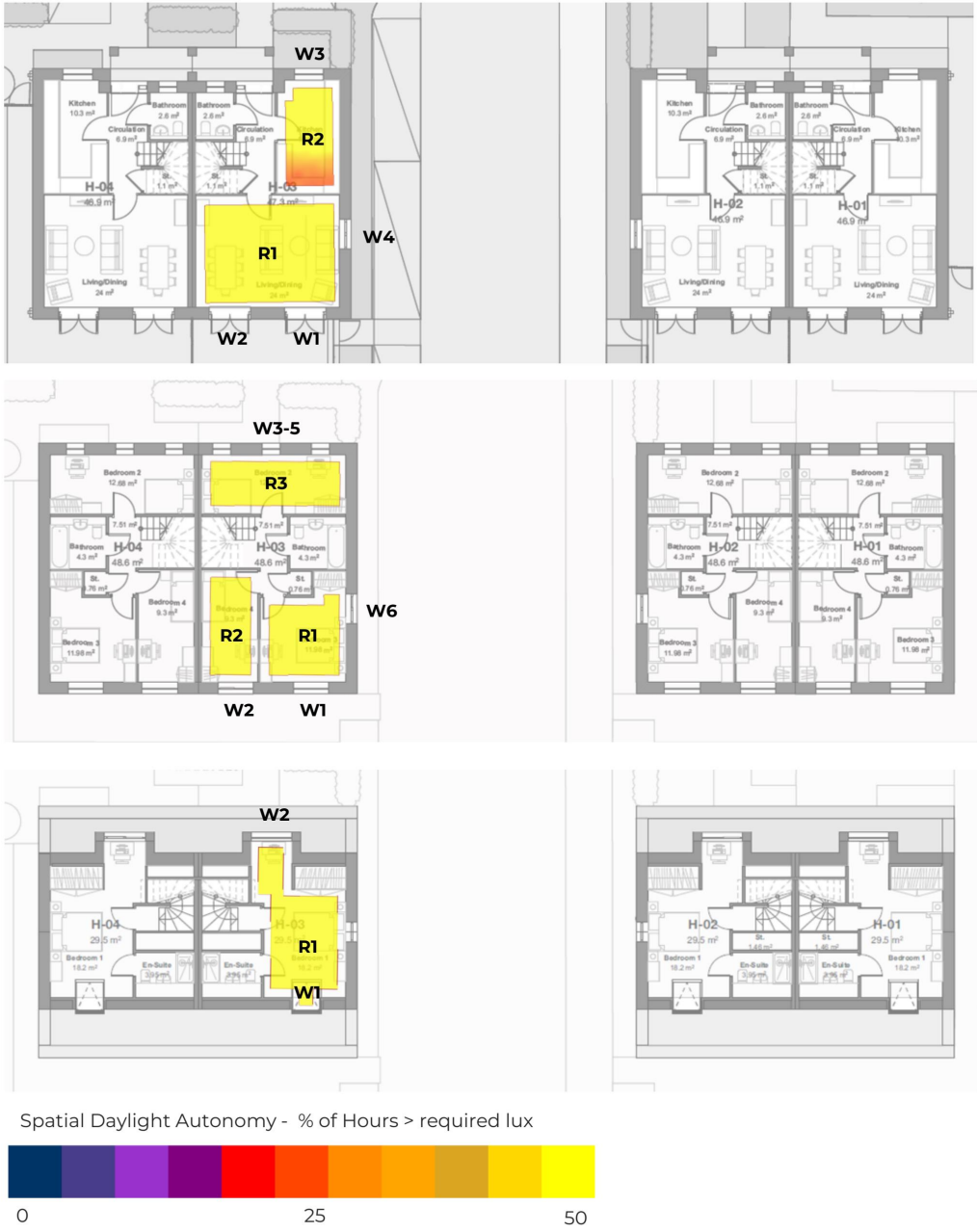
Figure 6. Spatial Daylight Autonomy (SDA) results for sample of House Type 2 (top: ground floor, mid: first floor; bottom: second floor), (with window and room references).
