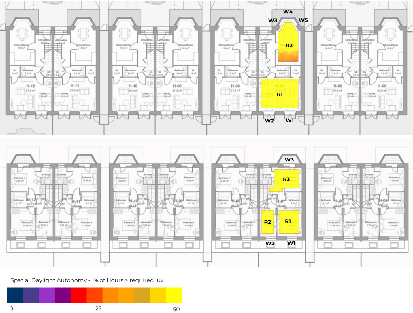
Figure 5. Spatial Daylight Autonomy (SDA) results for sample of House Type 1 (top: ground floor, bottom: first floor), (with window and room references).
