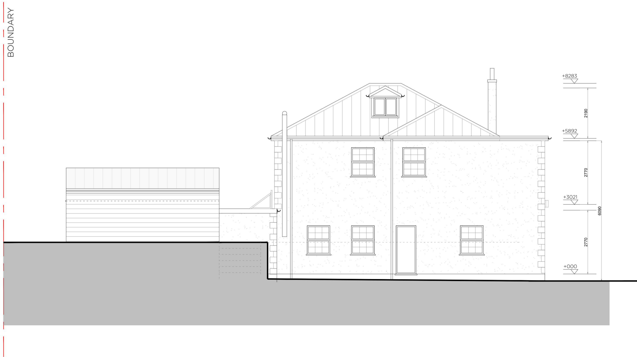
EXISTING East Elevation 1:100 @ A1 / 1:200 @ A3
