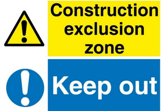
Figure 7. Example of suitable signage to be attached to protective fencing to create 'Construction Exclusion Zone'.
