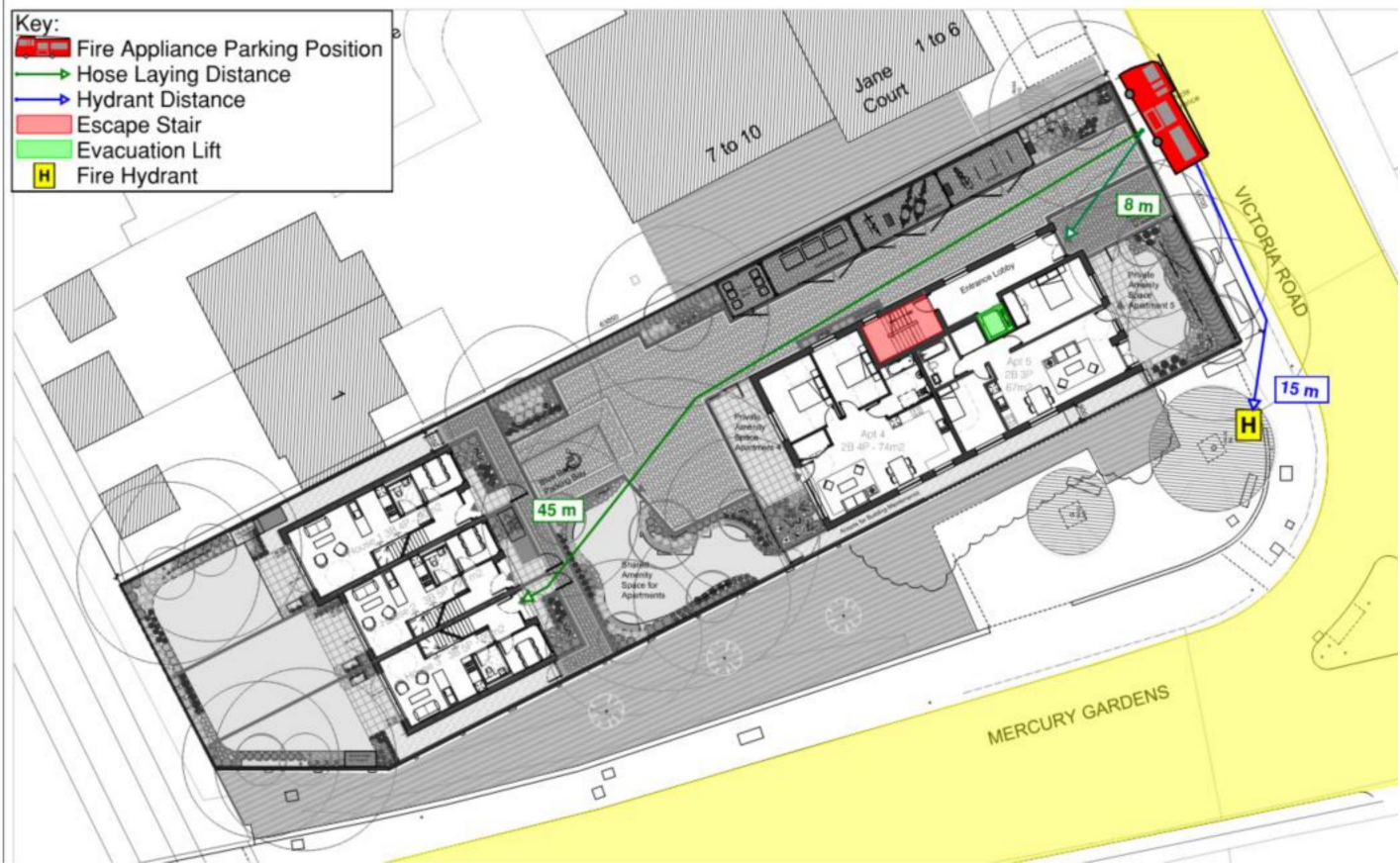
Fire appliance access, hydrant location, hose laying distances to apartment and terraced housing entrances.
