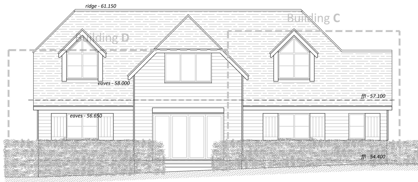
Rear (South Facing) Elevation 1:100
