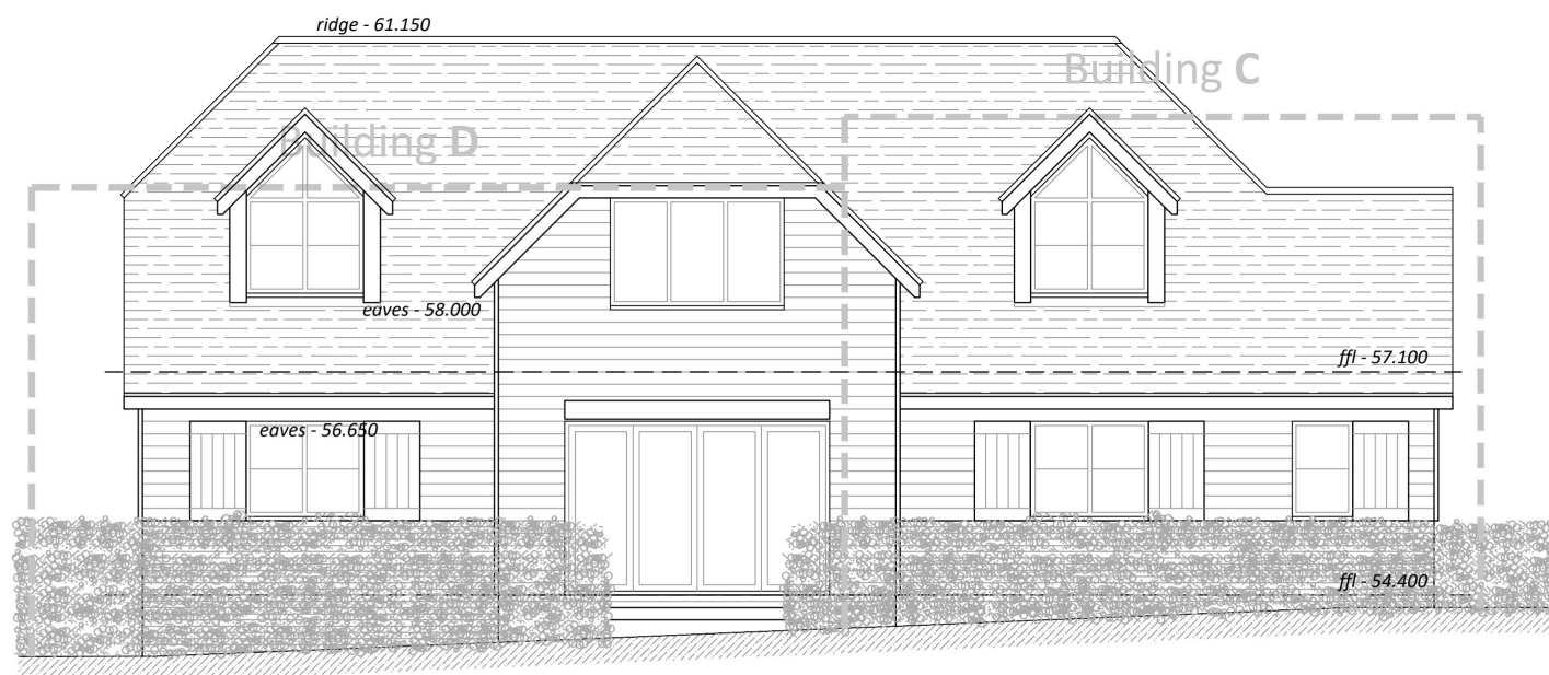
Rear (South Facing) Elevation 1:100
