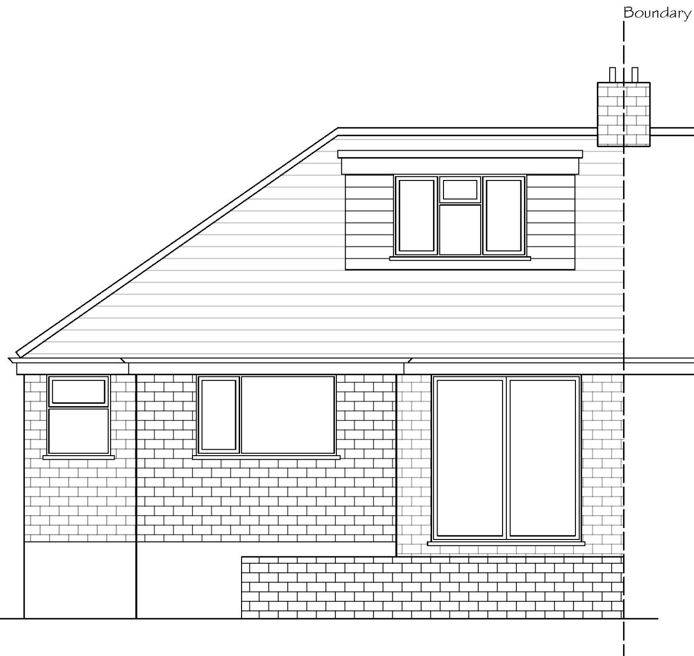
EXISTING REAR ELEVATION
