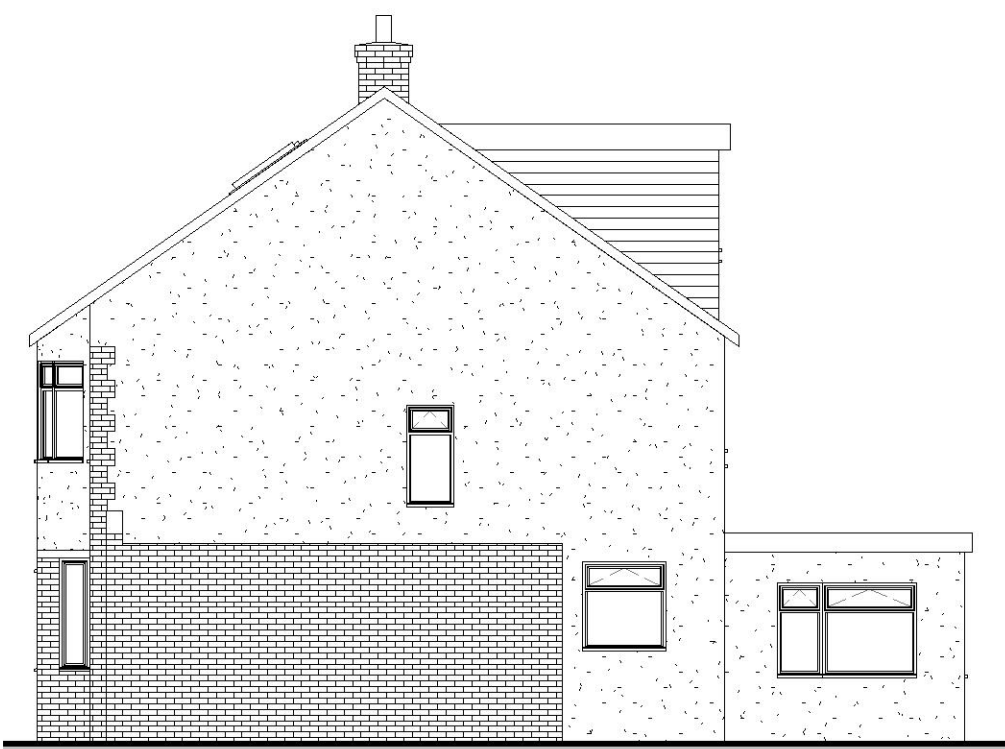
EXISTING SIDE ELEVATION 1 NO. 73 1 : 100
