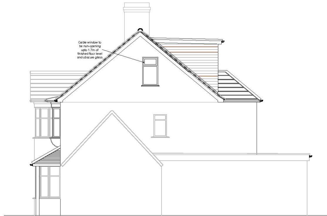
PROPOSED SIDE ELEVATION scale 1:100 at A1
