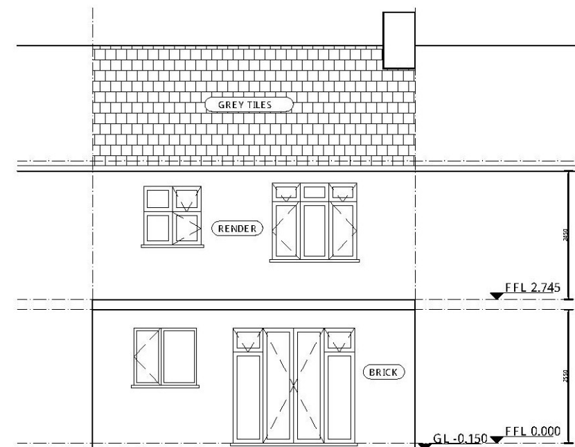
EXISTING REAR ELEVATION
