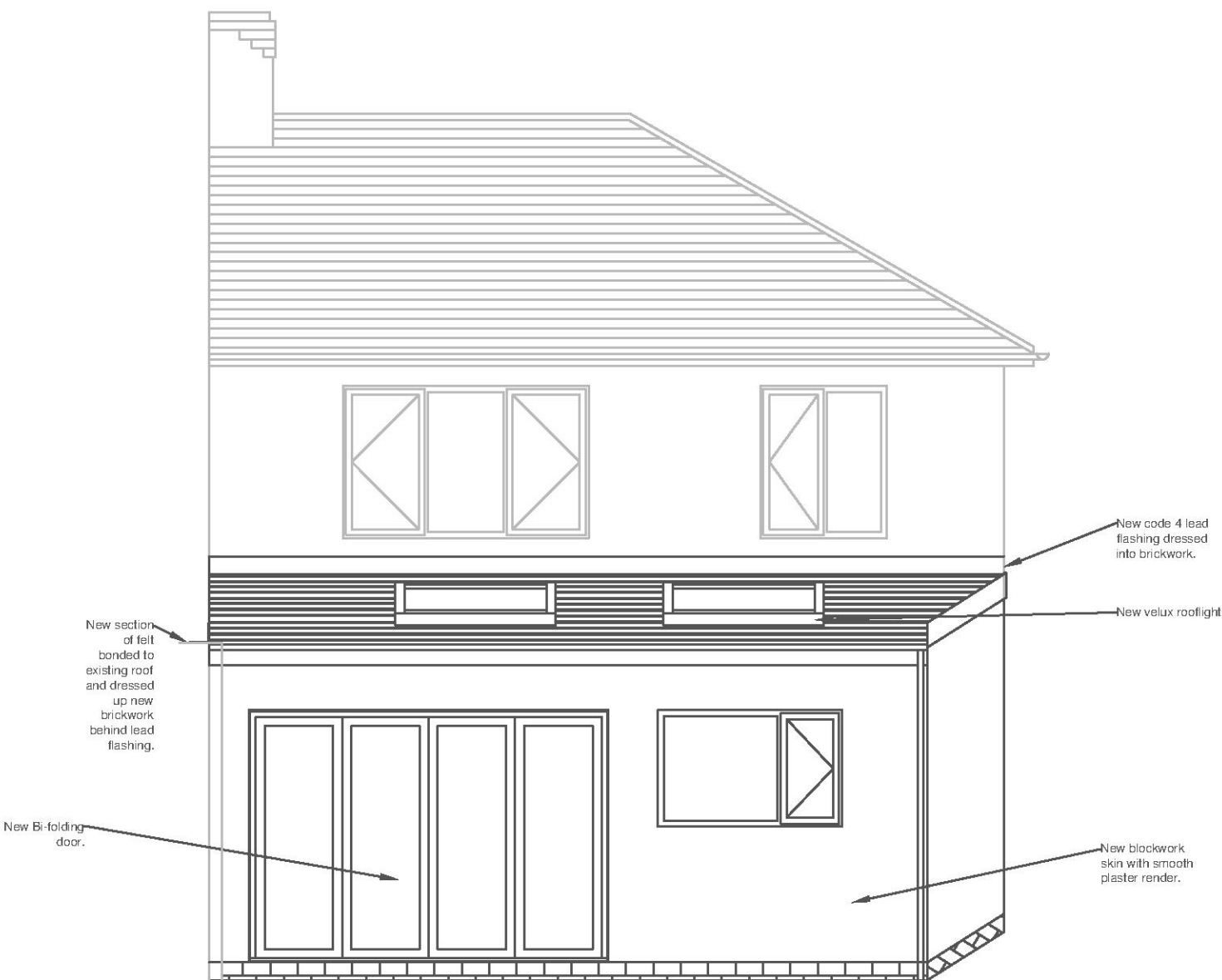
East Elevation (Rear)
